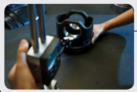
Cylinder liner dimensional control includes dozens of critical specifications, including inside and outside dimensions, flange specifications and oring groove size checks, which is accomplished through tools such as a CMM, height gauge, hardness testor and surface analyzer.
