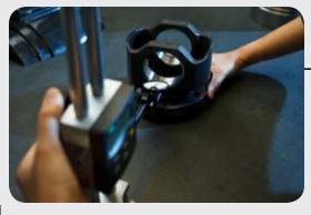
Cylinder liner dimensional control includes dozens of critical specifications, including inside and outside dimensions, flange specifications, and o-ring groove size checks, which is accomplished through tools such as a CMM, height gauge, hardness testor, and surface analyzer.
